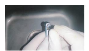
3. After cleaning, dry the spray nozzle by the three-purpose gun or similar way.
